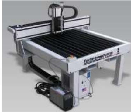
Figura 3: Corte plasma CNC [8].
